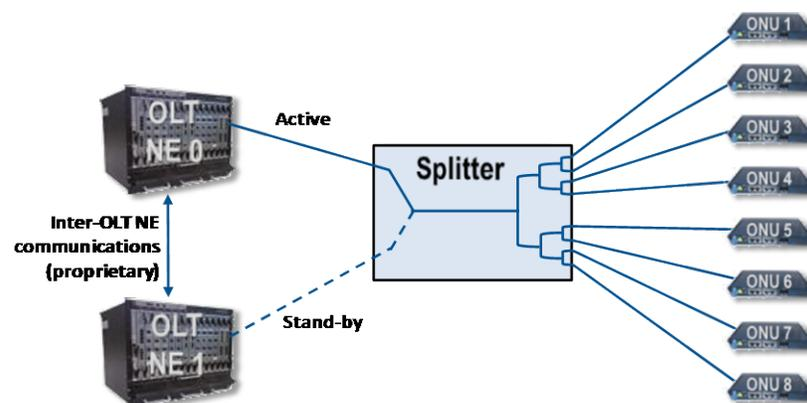
**Figure 3.** PON Type B Redundancy Example Utilizing Distinct OLT NEs
